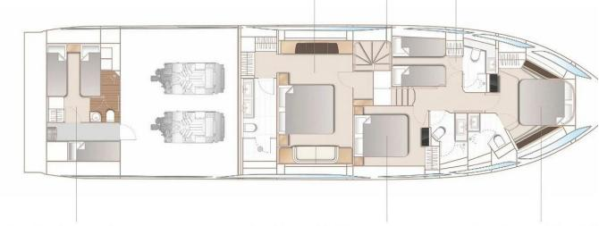
Crew Cabin with access from transom door, access to engine room, two single beds with storage below, wardrobe with shelf, mirror, storage lockers, opening porthole and venetian blind, individual berth lights, fited carpet and en suite bathroom
