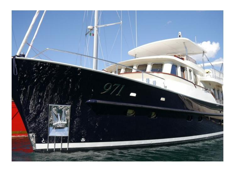
Expedition yacht De Alm Delfino 72 was built at the Dutch shipyard De Alm in 2013. The displacement hull is 22.5 meters. The yacht is powered by two Iveco engines and has a cruising speed of up to 8.5 knots. Her lower deck space has three spacious cabins for up to 6 guests and additional space for the crew cabin. Spacious main deck and flybridge spaces make this vessel a great option for travelling with a large group of guests. The yacht is in great condition and is located in the Montenegro.
